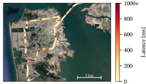
Fig. 4. Cellular network latency of a 5G connection while driving through a route in San Francisco frequented by Waymo and Cruise AVs.
